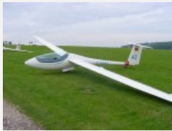
Schleicher ASW 27 An aircraft with shoulder wing, no engine and made of plastic
