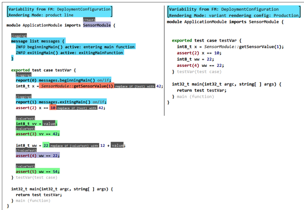
Figure 21.9: Left : A C program with product line annotations. Right : The program rendered in the Production variant. Note how the program is "cut down" to include only those parts that are part of the variant, even in the editor.
